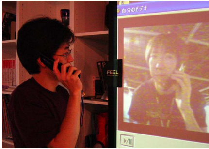
Figure 8: Extensible mobile phones: During a mobile phone conversation (1), user walks up to nearby computer display and makes a connection between the phone and the display (2). The IP addresses and a session key is transmitted over the mobile phone connection (3), displays in front of the phone talkers become a shared screen (4).
