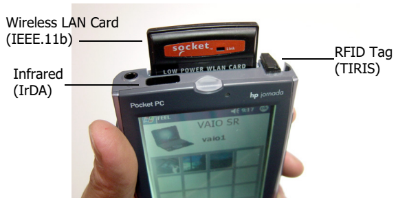
Figure 3: An example of enhanced PDA. Two proximal interaction channels (RFID tag and infrared beaming) are available in combination with normal wireless LAN.
