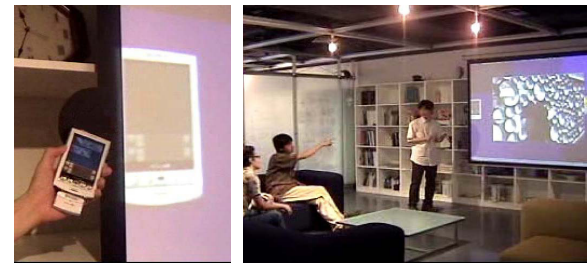
Figure 6: A presenter attaches his/her PDA to the presentation screen to make a connection between them. Then a user can select a file from the PDA display and show it on the presentation screen.
