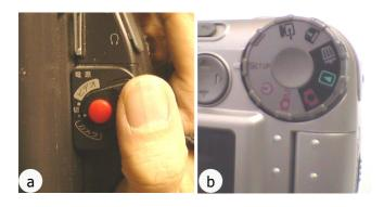
Figure 3: Tactile impressions reveal the state: (a) A camcorder switch with three states. A user can physically perceive the current state from the thumb position on the switch during operation. (b) A dial of a digital camera. In this example, the physical shape does not change so visual labels (hence, visual attention) are needed to know the current state.
