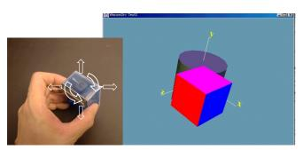
Figure 10: MDOF movement of the ToolStone can be mapped for 3D object control.
