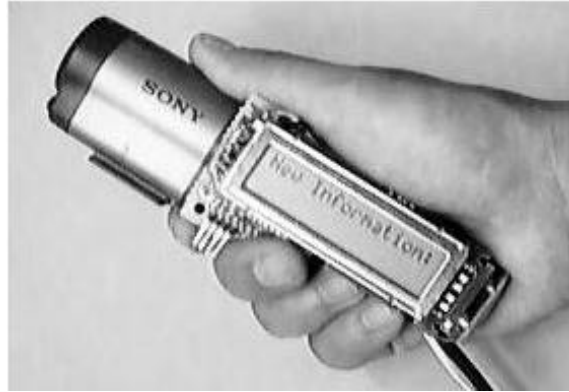
Fig. 8. A prototype data picking wand
